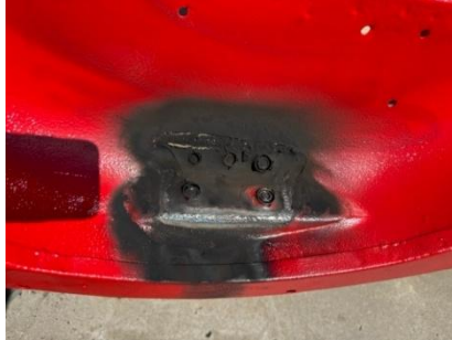
Damage to the underseal
