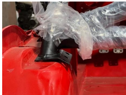
Gaps between feet and Wheel Arch
