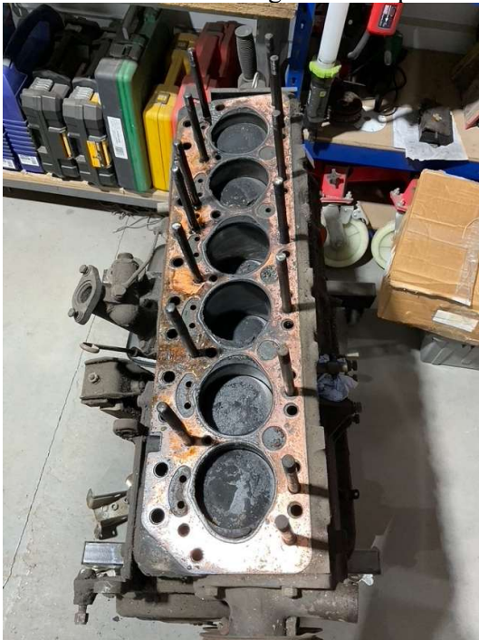
Carbon build-up on pistons and bores.
