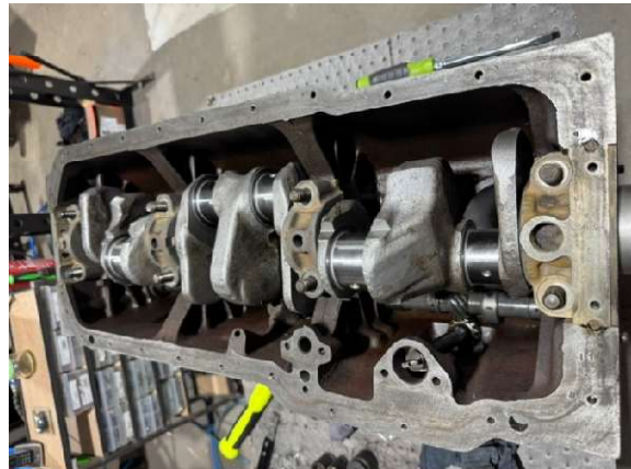
New main bearings and Crank during the rebuild.
